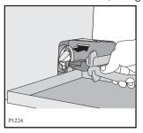
when no more water comes out, unscrew the pump cover, using a pliers, and remove the filter.
